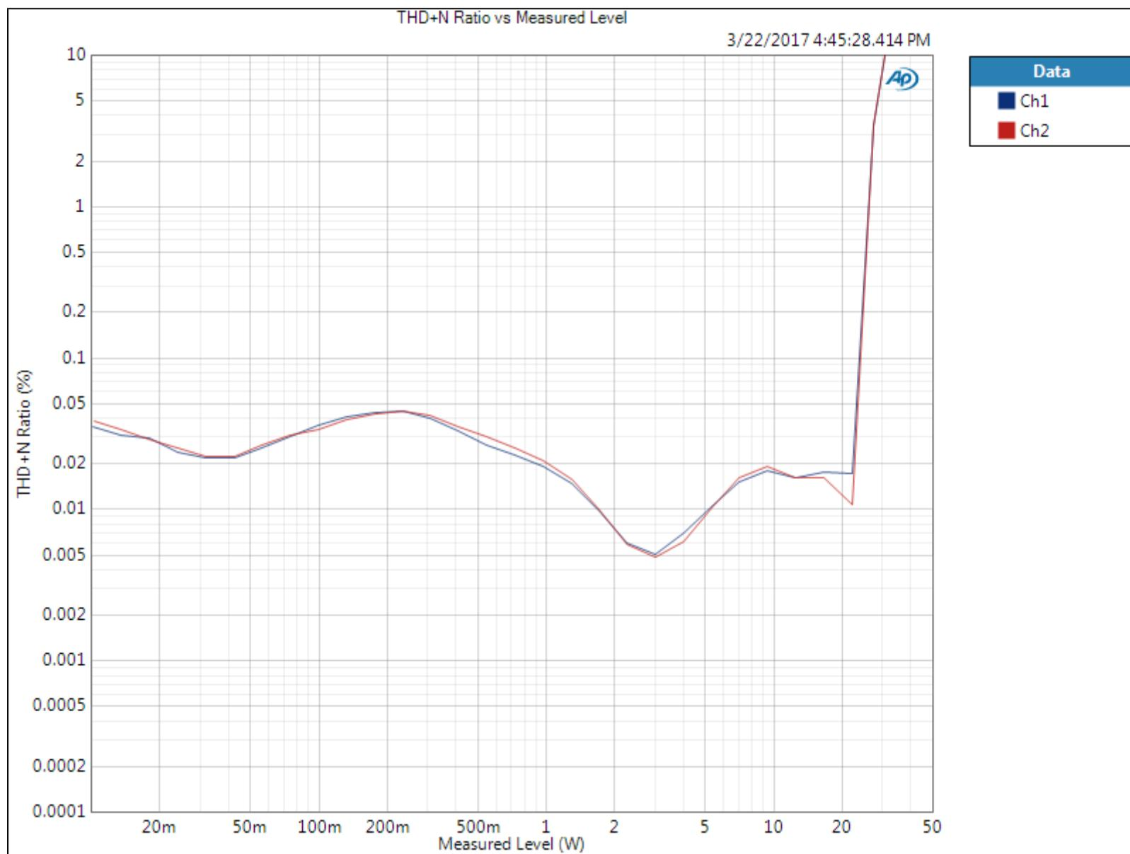
PVCC=19V; Gain=20dB, Load=8R;f=1kHz
