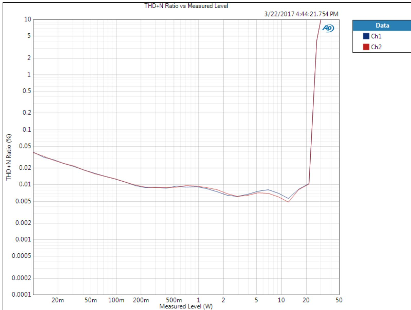
PVCC=19V; Gain=20dB, Load=8R,f=6kHz
